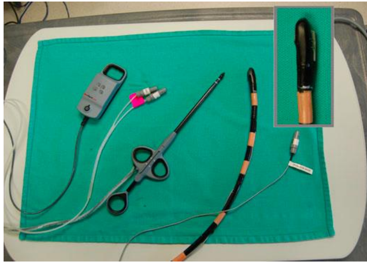
Figure 4.3: NeoChord DS1000 outfitted with tracking sensors (left) and TEE probe with sensor on back (right and insert, top right). Devices rest on the NDI Aurora tabletop magnetic field generator.
