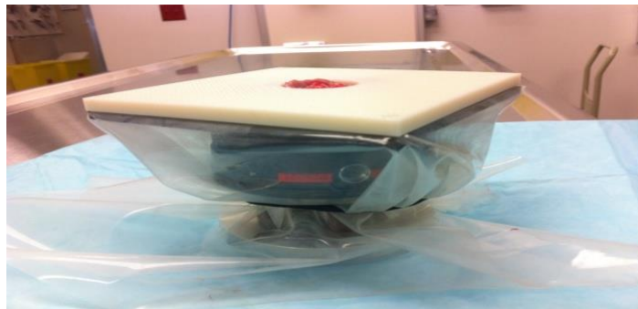
Figure 3.1: Mitral valve annuloplasty test bed. The tissue test bed consists of an excised porcine mitral valve mounted between two custom designed plates that firmly clamp the cardiac tissue along the outer edge of the annulus. The plates and valve are mounted on a six-axis force/torque sensor (ATI Industrial Automation, Apex, NC).
