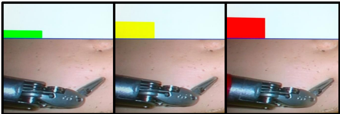
Figure 3.4: Visual force feedback, as shown to subjects. This figure shows the visual force feedback for the left surgical arm. Both colour and size denote the magnitude of the force applied by both the right and left arms. Green denotes the range of force/tension below the threshold required for a tight knot (under 4N). Yellow denotes the range sufficient for a tight knot (4-6 N). Red denotes force that may damage the tissue or break the suture (above 6N).
